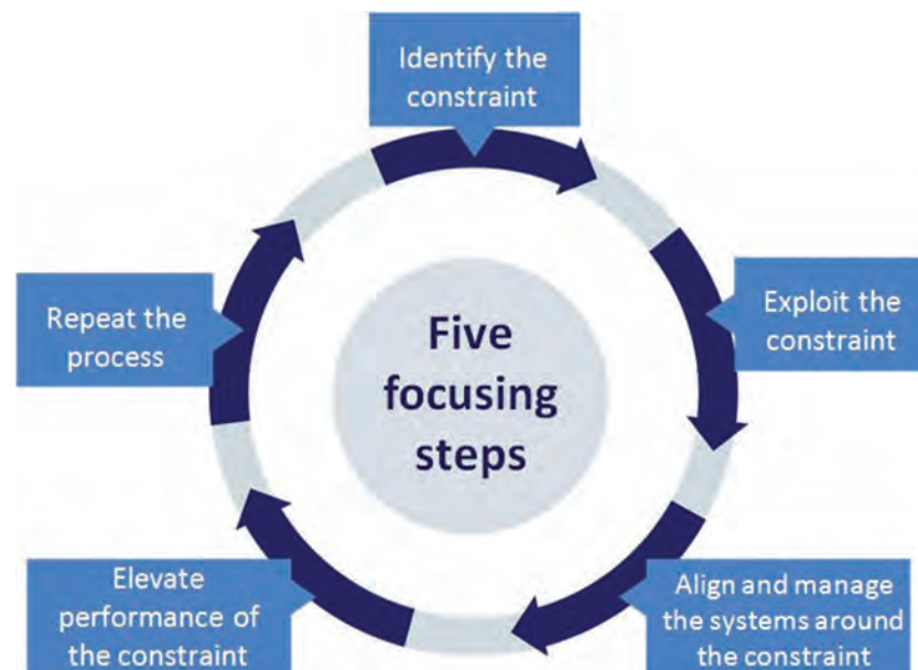
Figure 2: The theory of constraints uses a process known as the five focusing steps to identify and eliminate constraints (ie bottlenecks)
